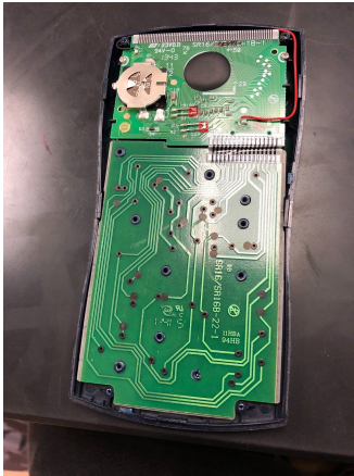
Photo of the circuit board inside a TI-30 calculator
